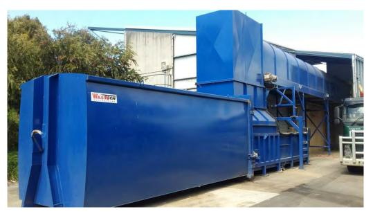
The installation of Council's new compactor means that transport costs to Port Latta have been reduced due to less volume of trash due to compaction. Other cost reductions as a result of the new compactor include the number of trucks and skips required to cart rubbish, less man hours to cart rubbish, less down time more efficient use of Council resources.
