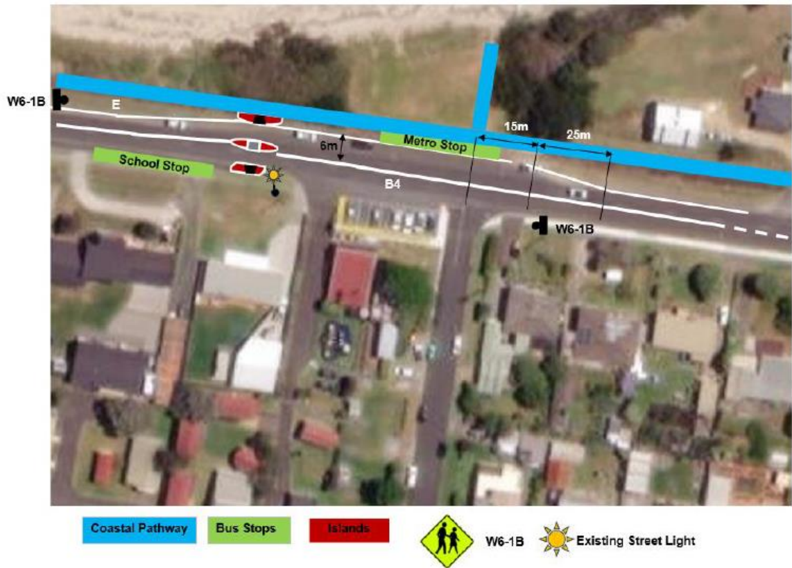
Figure 32 Old Bass Hwy / Dart Street junction improvement
