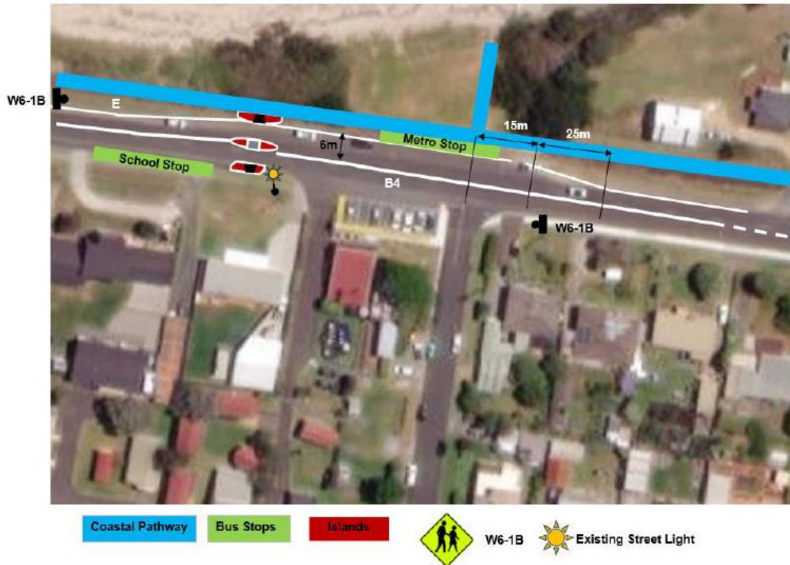
Figure 32 Old Bass Hwy / Dart Street junction improvement
