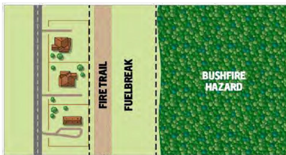
Figure 2: Fire trail placement within a protective (Class 2) fuel break
