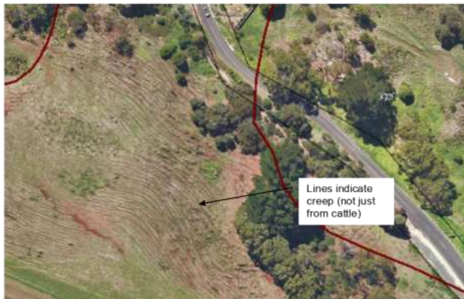
Photo 6. Evidence of creep on slopes above Port Road
