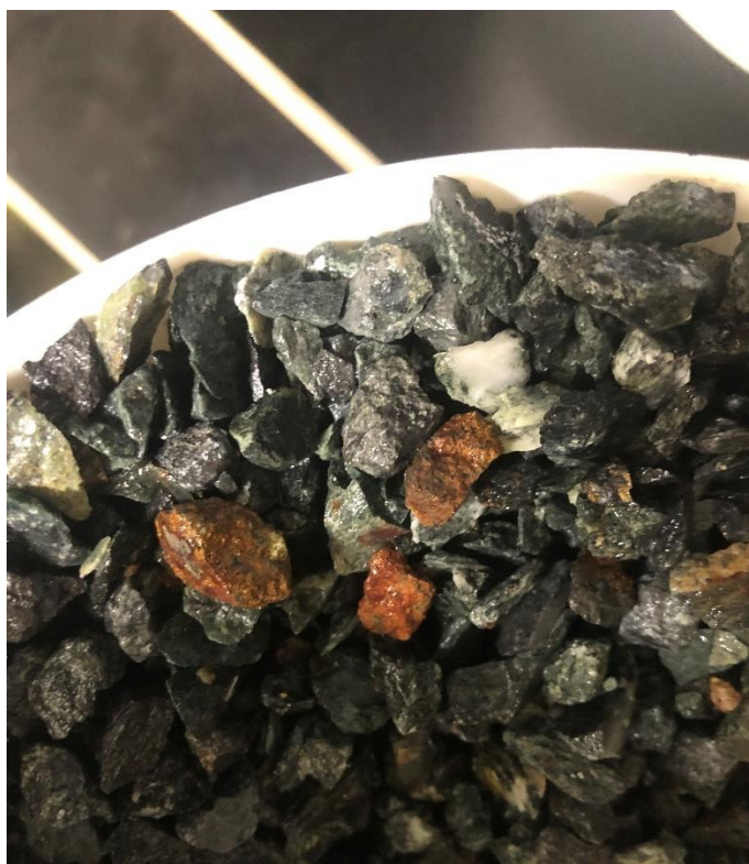
Figure 33. Example of visual oxidation- Column 2 post kinetic trial.
