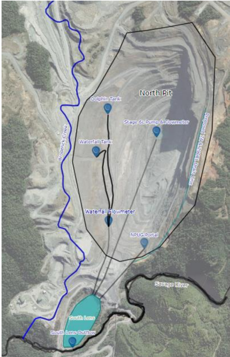
Figure 15 - Existing North Pit water management
