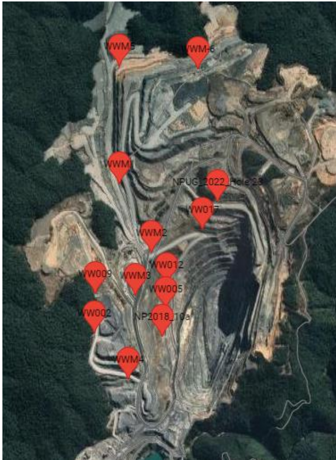
Figure 27 – Fixed vibrating wire piezometers (VWPs) locations
